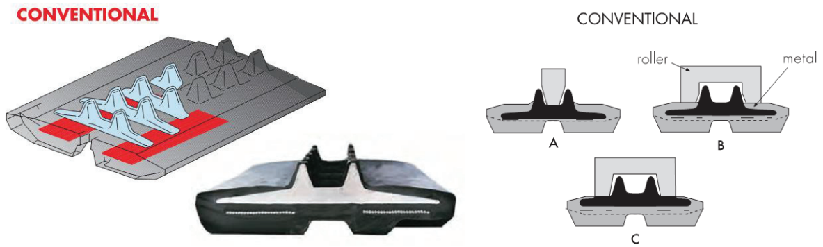
Fig. 2 Construction of the rubber track with a metal core and the steel cords (left); Types of track construction for the different options, A – Internal side of the track, B - External side of the track, C – External side of the track with the metal trackline. [5]
