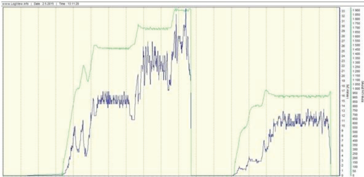
Fig. 3 A dependency of an electric current consumption at a rotor speed. The vehicle is a helicopter series 500. The green line is the rotor speed. The blue line is the current [3]
