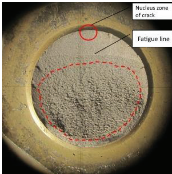
Fig. 4 Appearance of the fracture under the head of bolt No. 18-3 [10]
