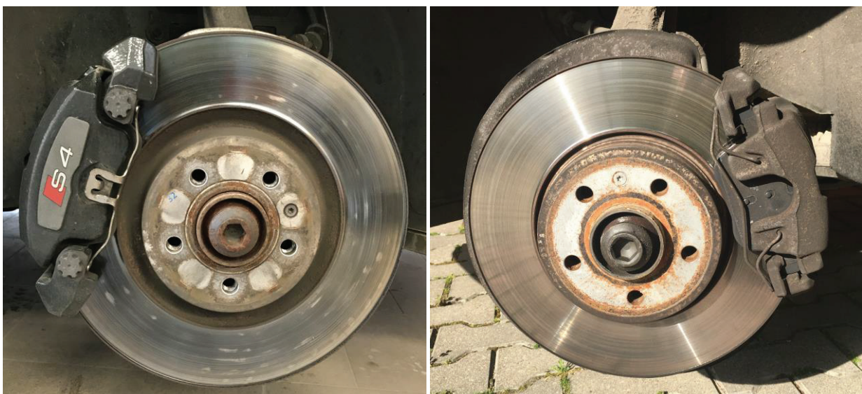
Fig. 3 The view of brake calipers in Audi S4 \varnothing 345 [left] and Audi A4 \varnothing 330 [right]
