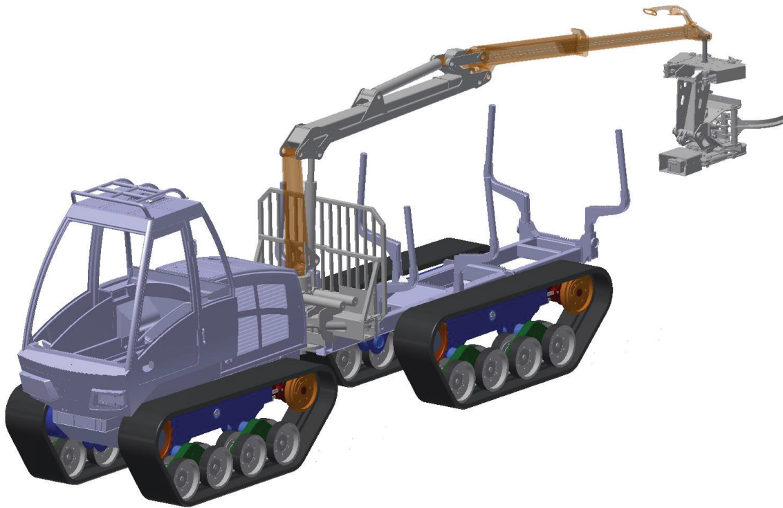
Fig. 9 The virtual prototype of the forwarder with a tracked chassis
