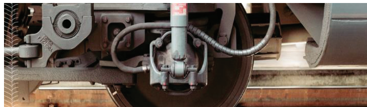
Fig. 1 Monitoring of hot axle box bearing temperature by on-board monitoring system
