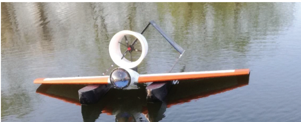
Fig. 16 Rescue UAV (technology demonstrator) with the propulsion system designed on the basis of the experimental and numerical studies, Materials Technology Student Research Circle, Polish Air Force Academy, Dęblin, photo T. Muszyński
