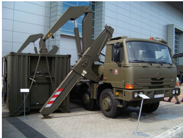
Fig. 2 An example of a container carrier on TATRA 815 8×8 equipped with a side container loading and unloading [1]
