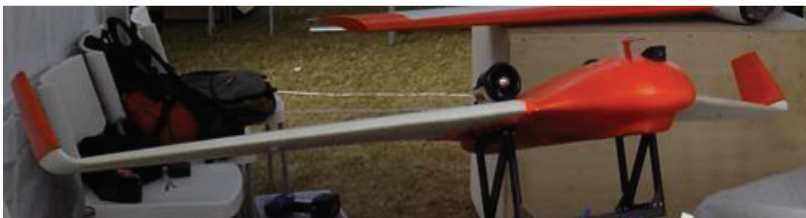
Fig. 1 Rescue UAV with EDF turbine propulsion system manufactured by AeroaAtena and FlytechUAV consortium, photo T. Muszyński
