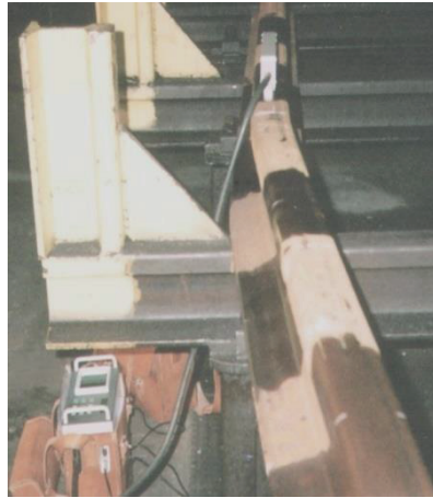
Fig. 1 Measurement of residual stress with DEBRO instrument
